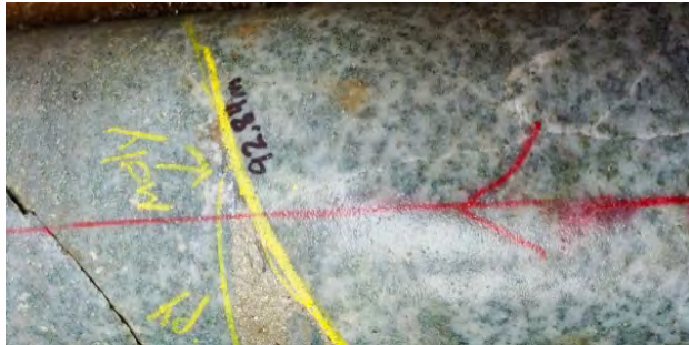
Early iron and molybdenum sulphides in dioritic endoskarn Hole ZM17010, 92.84m
