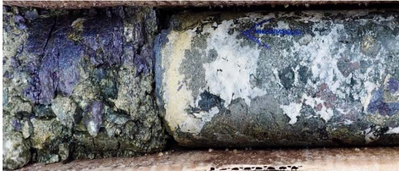
Figure 2: Bornite mineralisation in garnetiferous skarn, drill hole ZM17010, 179.4m
