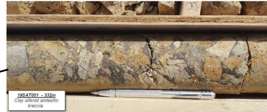
19SAT001 at 332m depth. Argillic alteration overprinting brecciated andesite.
