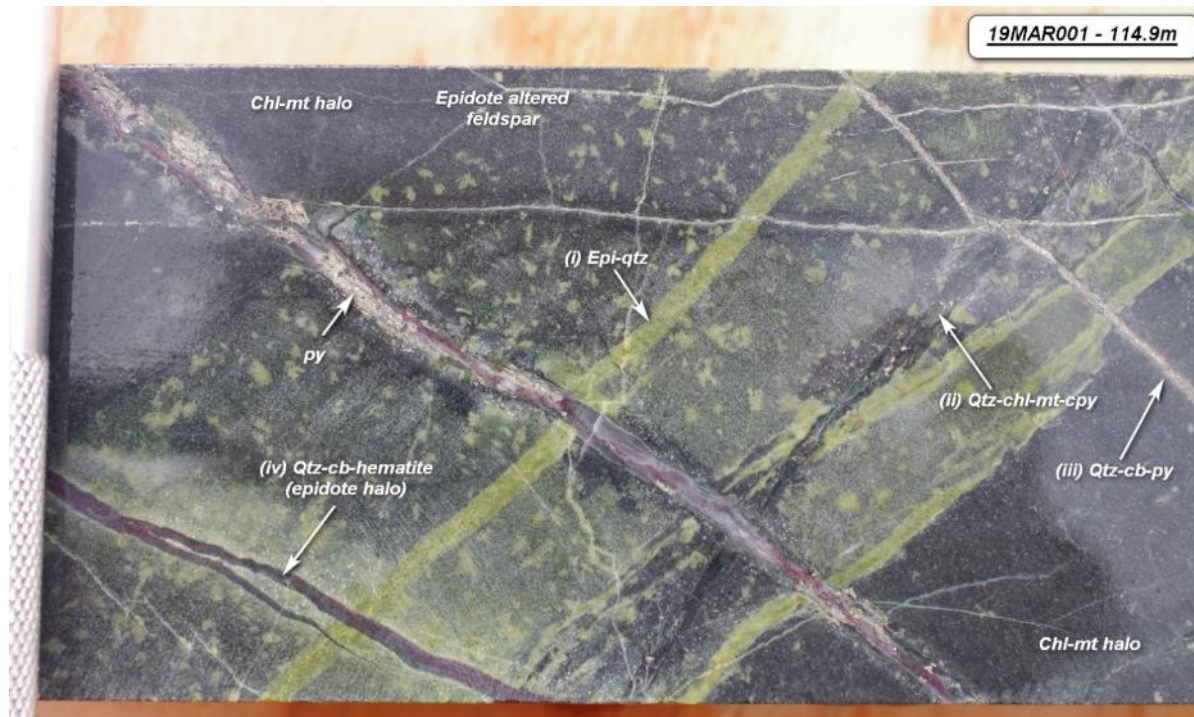
19MAR001 at 114.9m depth. Early phase (i) epidote-quartz veins with epidote haloes overprinted by three later phases of veining including (ii) quartz-chlorite-magnetite-chalcopryite, (iii) quartz-carbonate-biotite and (iv) quartz-carbonate-hematite.
