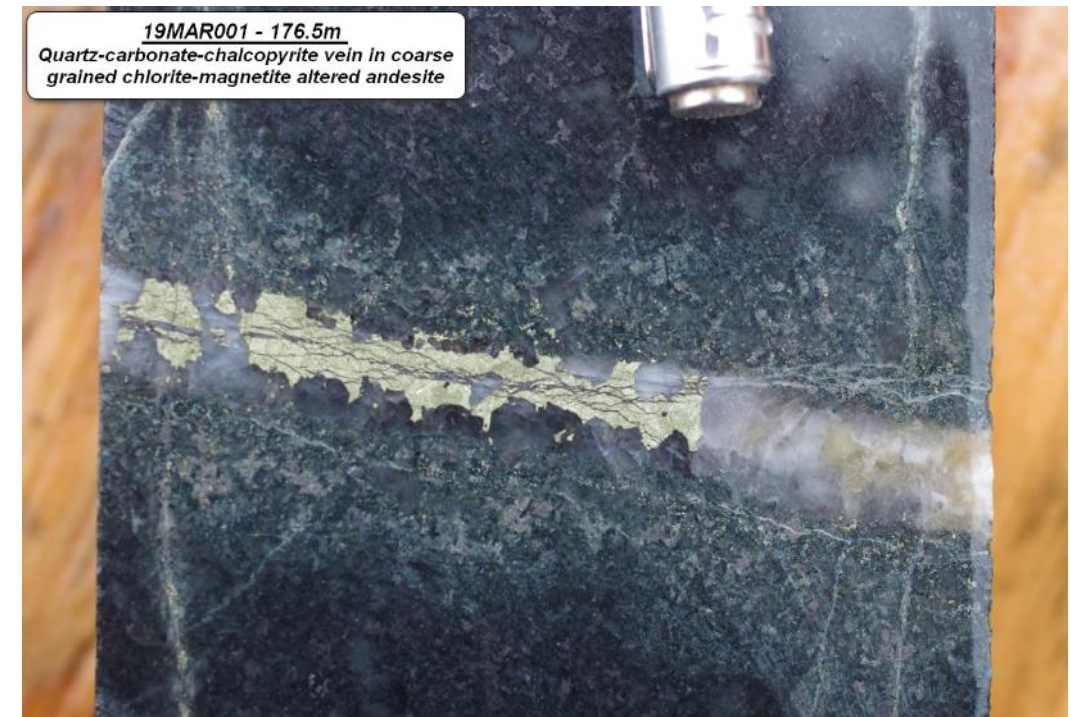
19MAR001 at 176.5m depth. Quartz-carbonate-chalcopryite vein with weak selvage of chlorite and sericite(?).
