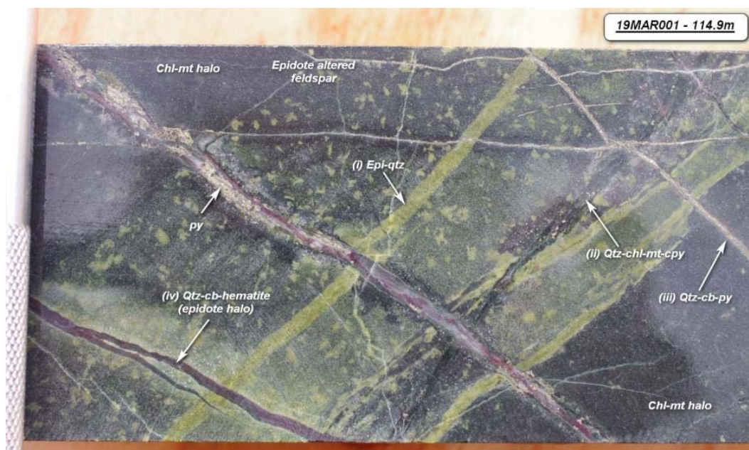
19MAR001 at 114.9m depth. Early phase (i) epidote-quartz veins with epidote haloes overprinted by three later phases of veining including (ii) quartz-chlorite-magnetite-chalcopryrite, (iii) quartz-carbonate-biotite and (iv) quartz-carbonate-hematite.
