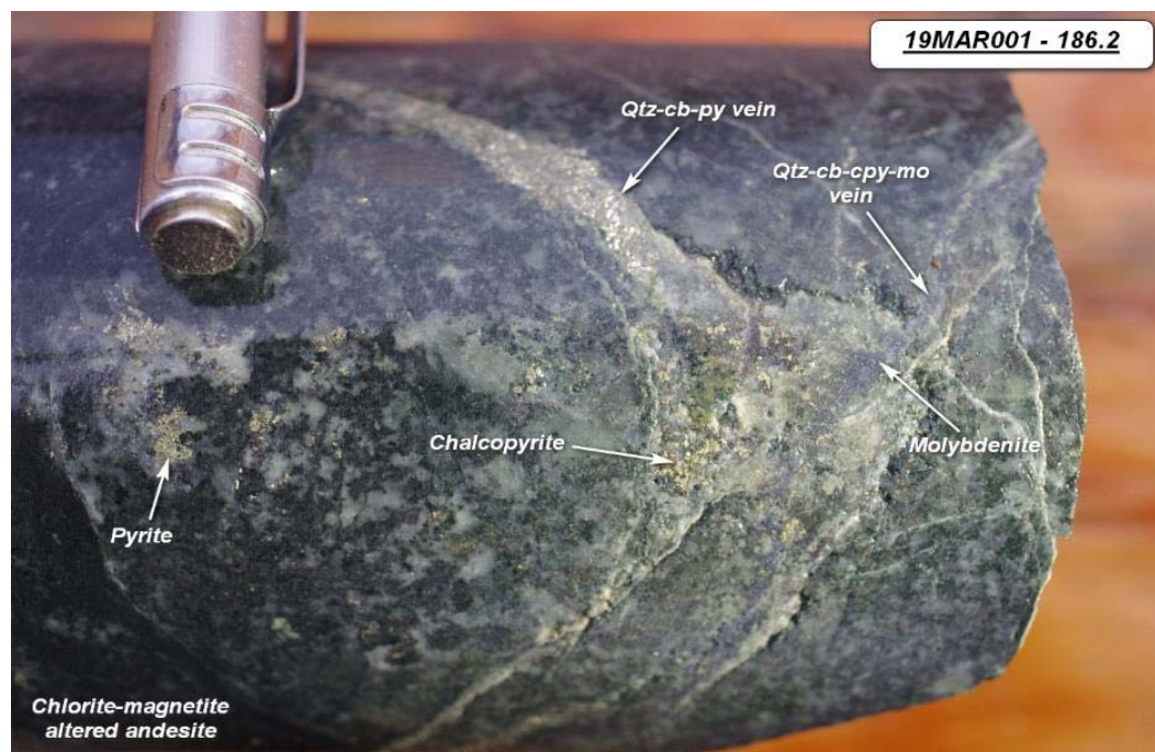
19MAR001 at 186.2m depth. Chalcopyrite and molybdenite in quartz-carbonate-pyrite veins.
