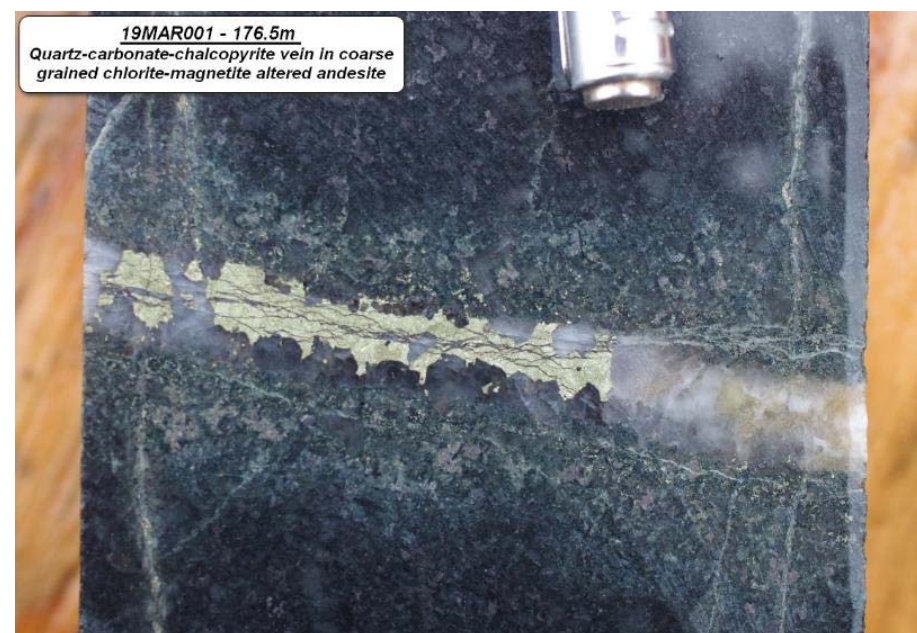
19MAR001 at 176.5m depth. Quartz-carbonate-chalcopryrite vein with weak selvage of chlorite and sericite(?).
