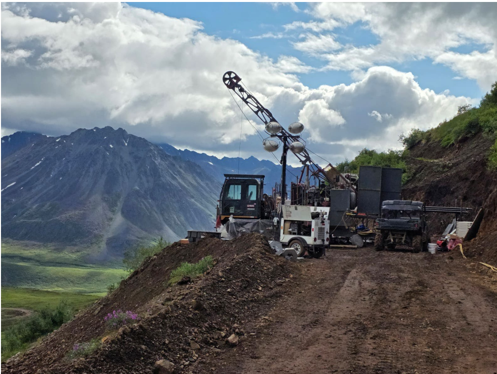
Figure 3. Diamond drill rig recently commenced oriented diamond coring at Caribou Dome (CD25-001)
